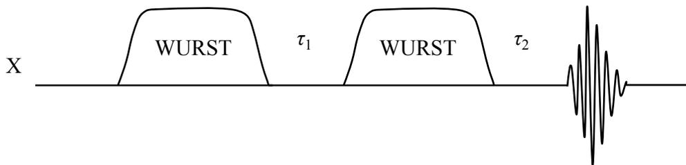
**Figure 2.17.** The WURST echo pulse sequence.
