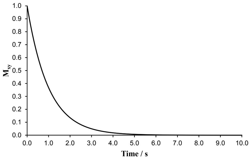
**Figure 2.13.** Spin-spin relaxation of nuclei with  $T_2 = 1.0$  s.
