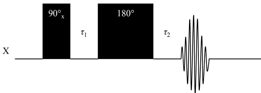
**Figure 2.15.** The spin echo pulse sequence.
