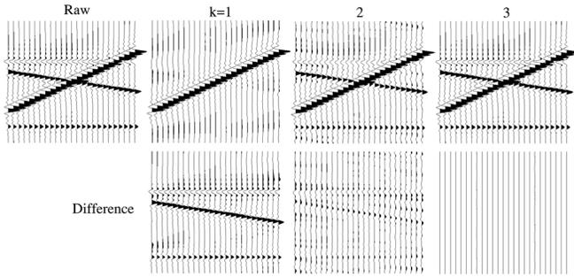
Figure 1: The exactness property. Eigen filtering is carried out with increasing values of  $k$ . Filtering with  $k = 3$  does nothing since it equals the number of distinct dips.
