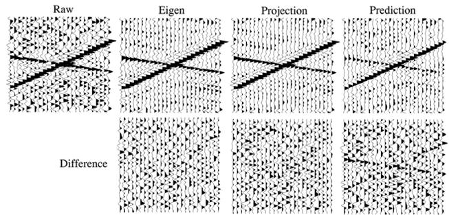
Figure 2: F-x eigen, projection, and prediction filtering on noisy artificial data. Eigen and projection filtering both show artifacts, although this does not tend to be a problem with real data.
