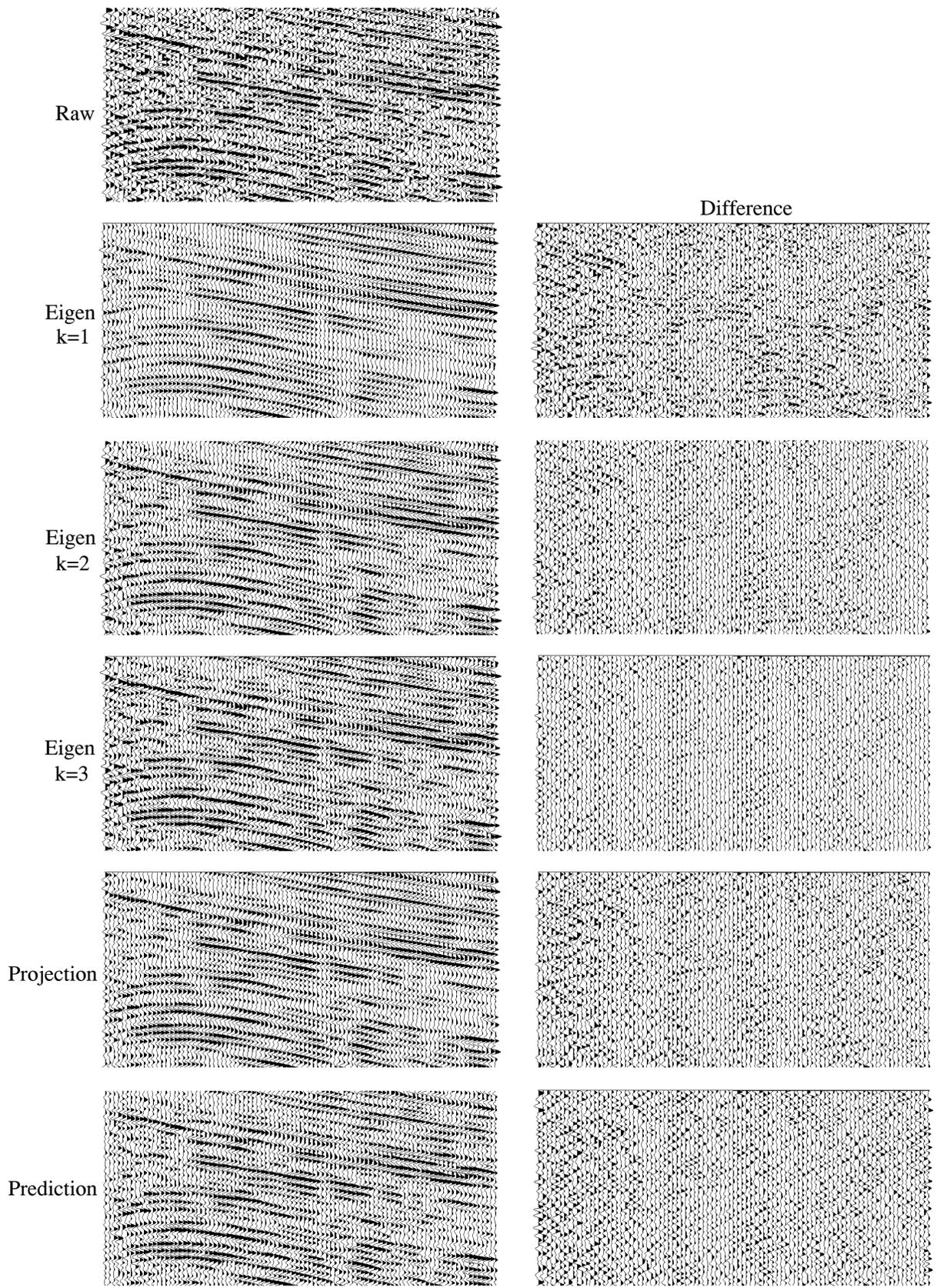
Figure 4: Noise suppression on real data using eigen, projection, and prediction filters. By adjusting  $k$ , eigen filtering can be tailored to almost any level of noise suppression.
